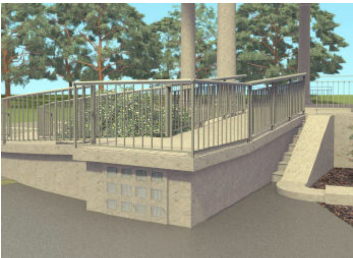
Detail view – Ramp construction at stairs. Skirt is shown recessed, with a door for storage beneath.
