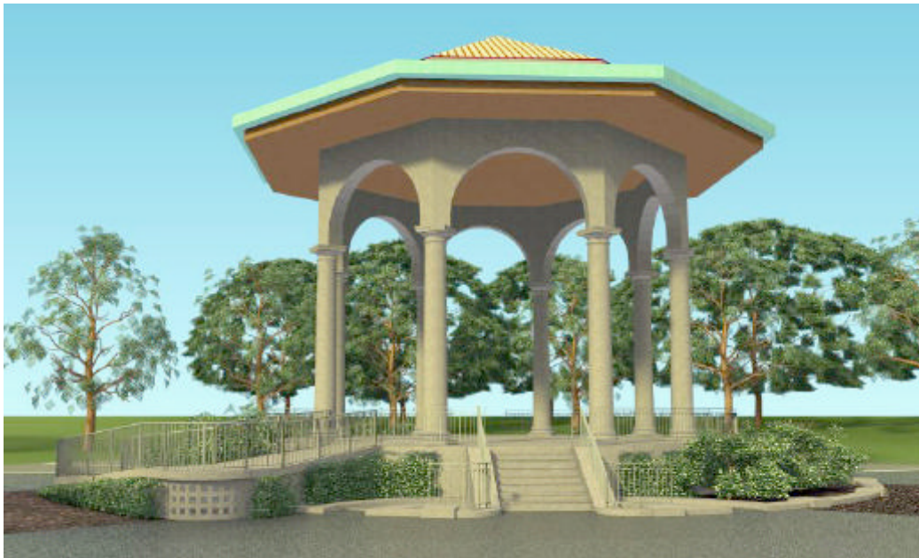
Option 13a – Ramp with round landing and recessed skirt, showing storage door and additional planting.
